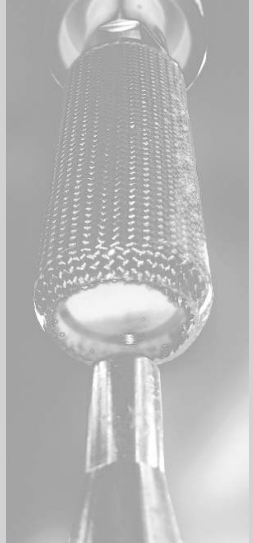
automatic ultrasonic solder nozzle cleaning
